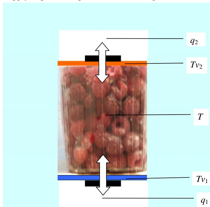
Fig. 1. Experimental scheme for determination of heat conductivity coefficient of frozen berries
