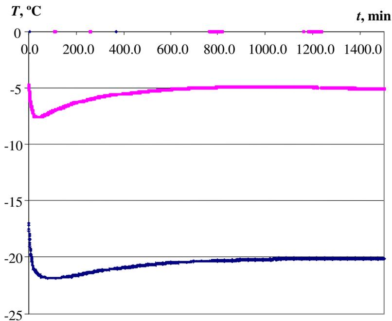
Fig. 3. Change of temperature  $T$  of raspberry sample surfaces during the process time  $t$
