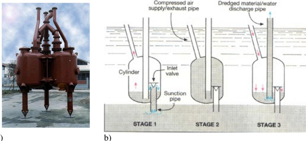
Fig. 2. Pneumatic suction dredge pump (a) [6], work cycle of the pumps (b) [8]
