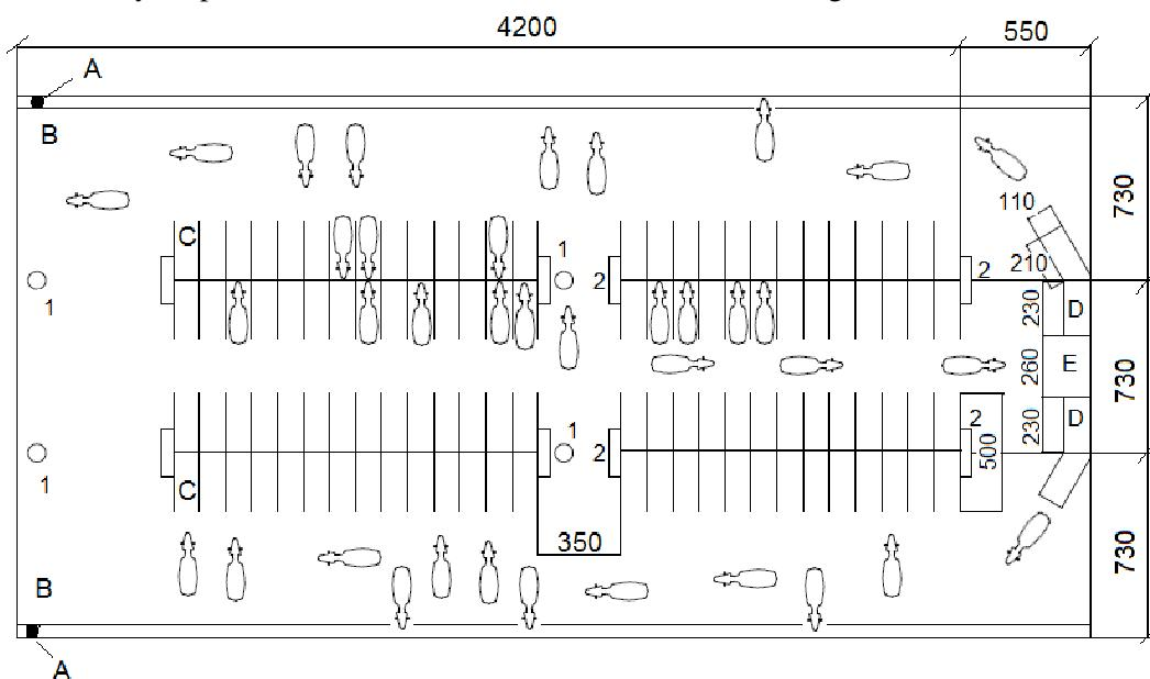
**Fig. 1. Layout plan of the free-type barn where the experiments are carried out (the sizes are in centimeters):** A – Forage line; B – Feeding area; C – Cubicles; D – Robots; E – Waiting area; 1 – Cow brushes; 2 – Troughs
