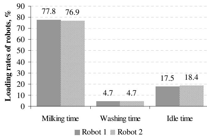
Fig. 5. Ratios of milking, washing and idletimes of the robots
