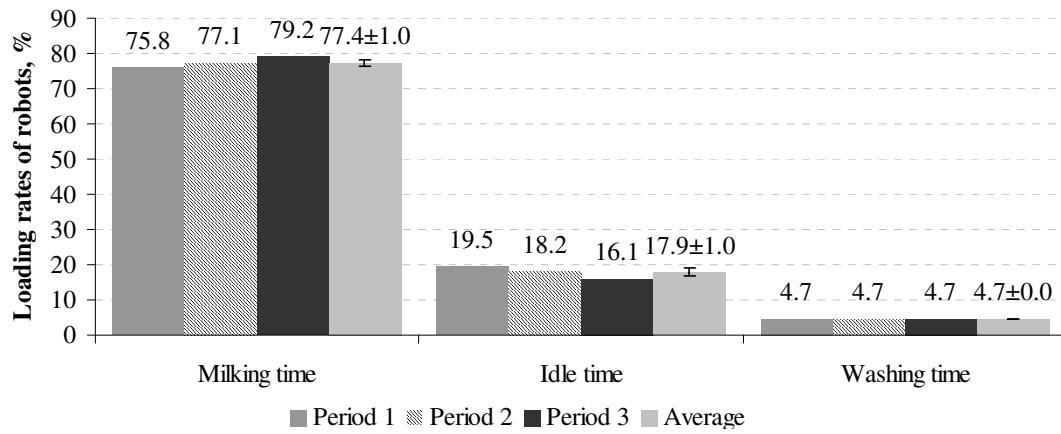
Fig. 4. Ratios of milking, washing and idle times of the robots in three periods
