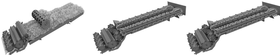
Fig. 2. Working mechanisms of Claas combine harvester: from left Mega 208, Lexion 600 and Lexion 770 [8]
