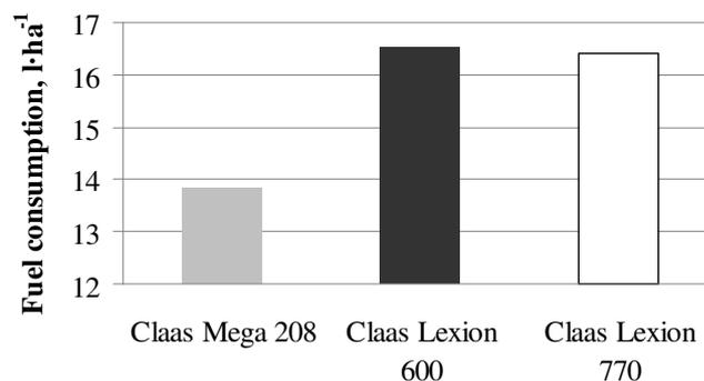
Fig. 4. Evaluation of fuel consumption – Claas Mega 208, Lexion 600 and Lexion 770 in winter wheat harvest
