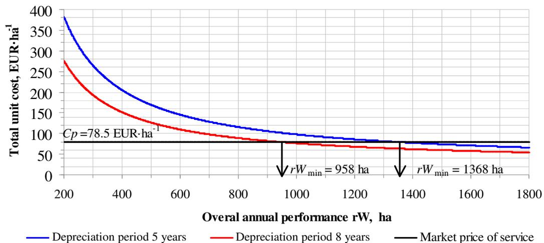
Fig. 8. Total unit cost dependence on annual performance of Claas Lexion 770 by different depreciation periods ( $C_p$  – average price of harvesting service)
