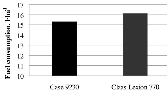
Fig. 3. Fuel consumption of Case 9230 and Claas Lexion 770 in spring barley harvest
