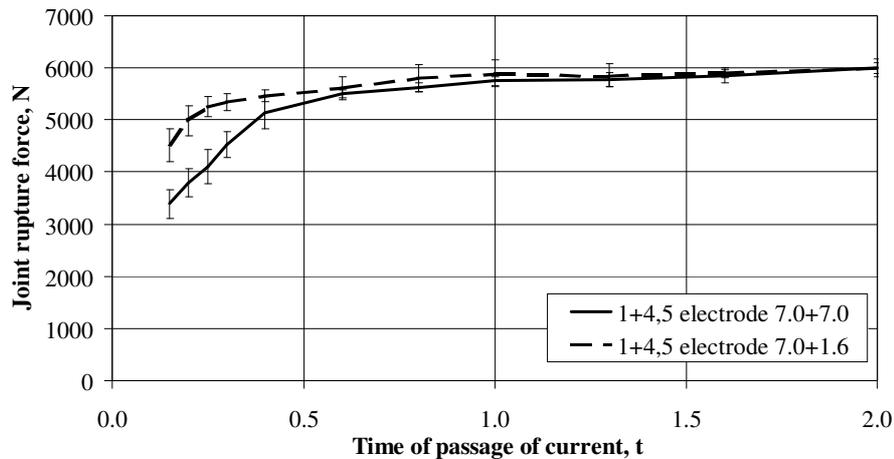
Fig. 5. Relation between rupture force and time of passage of current for sheets thickness 1 + 4.5 mm
