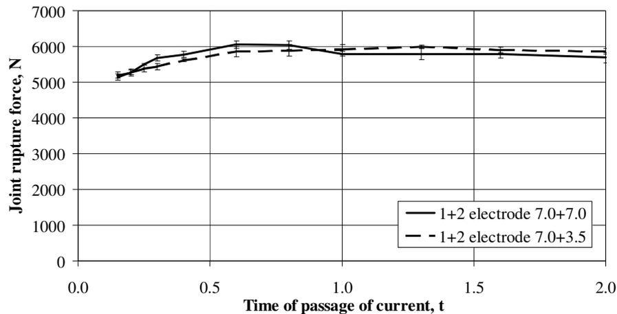
Fig. 3. Relation between rupture force and time of passage of current for sheets thickness 1 + 2 mm
