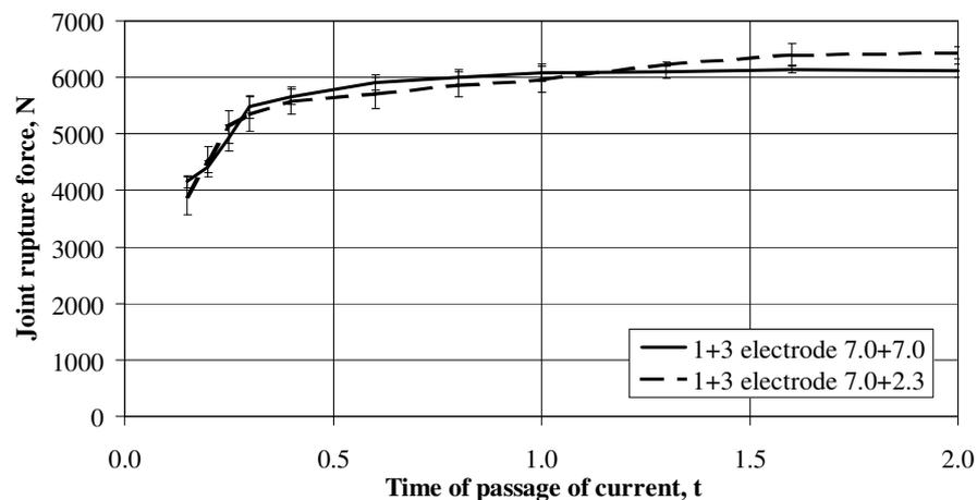
Fig. 4. Relation between rupture force and time of passage of current for sheets thickness 1 + 3 mm
