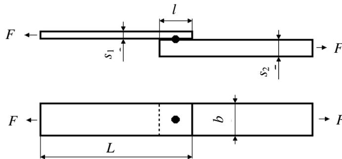
Fig. 2. Dimensions and shape of test assemblies
