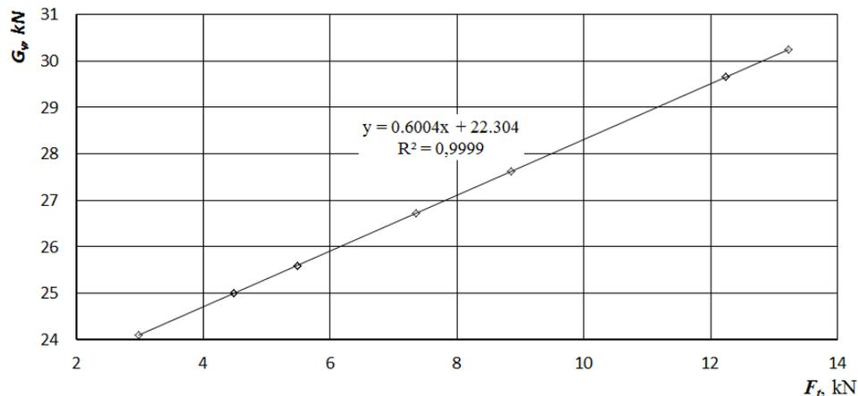
Fig. 1. Tractor "New Holland T5070" vertical load of the rear wheels  $G_v$  dependence on drawbar pull of  $F_t$
