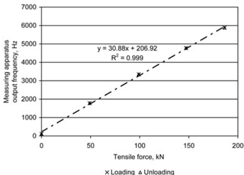
Fig. 4. Dependence of measuring apparatus output frequency on tensile force, load cell calibration curve
