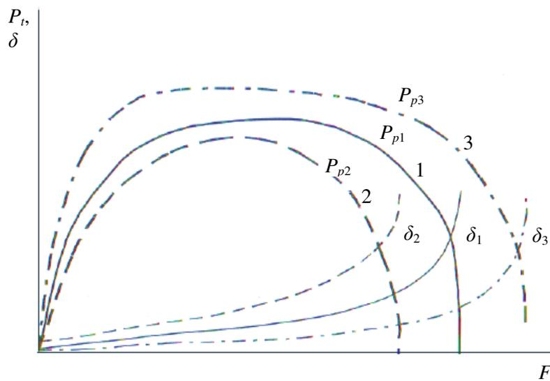
Fig. 1. Influence of ground to potential characteristics: 1 – stubble; 2 – soil; 3 – asphalt surface;  $\delta$  – wheelspin;  $P_p$  – potential pulling power;  $P_t$  – pulling power;  $F_t$  – tensile force [7]
