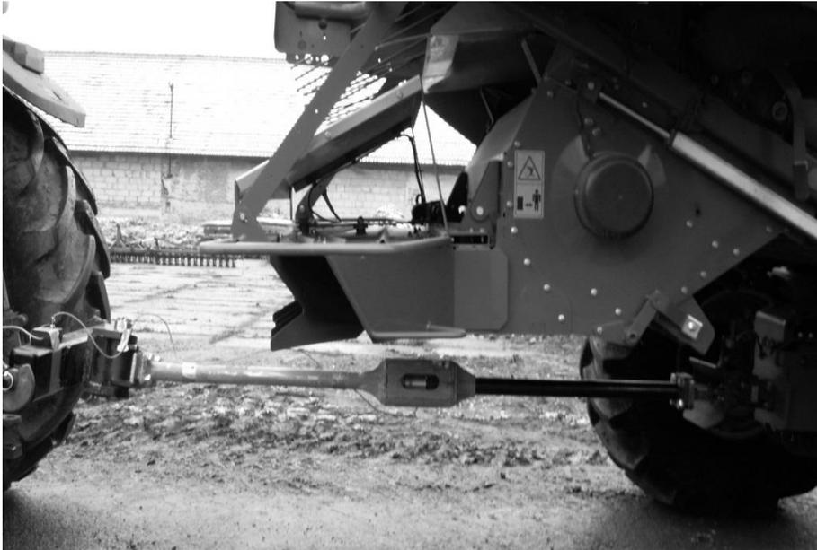
Fig. 3. Measuring equipment between combine harvester and tractor
