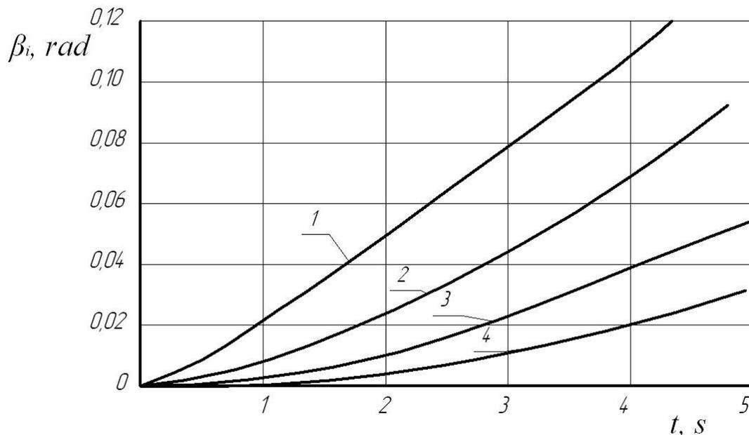
Fig. 3. Dependence of the turning angles of the trailed hemp harvesting aggregate (1 –  $\beta_1$ , 2 –  $\beta_2$ , 3 –  $\beta_3$ , 4 –  $\beta_4$ ) on time at  $\alpha = \pi/40$
