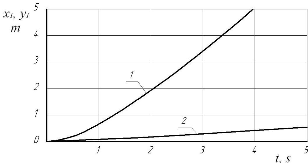
Fig. 2. Dependence of the path covered by the mass centre of the aggregating tractor on time in the direction of axis  $x$  (curve 1), axis  $y$  (curve 2), at  $\alpha = \pi/40$
