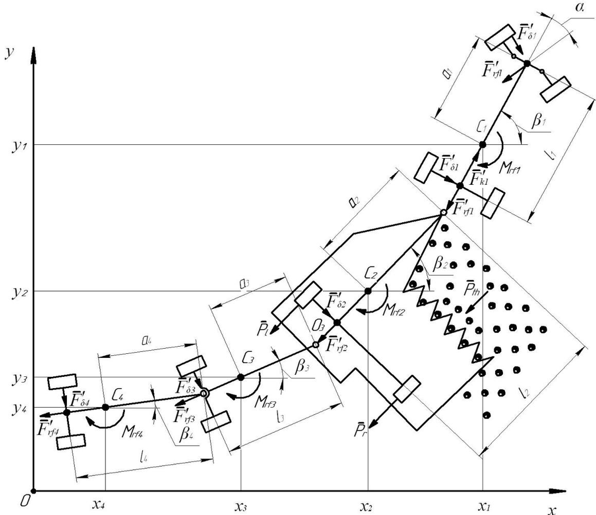
Fig. 1. **Equivalent scheme of the trailed hemp harvesting aggregate:** 1 – tractor; 2 – hemp combine harvester; 3 – hitch mechanism; 4 – trailer
