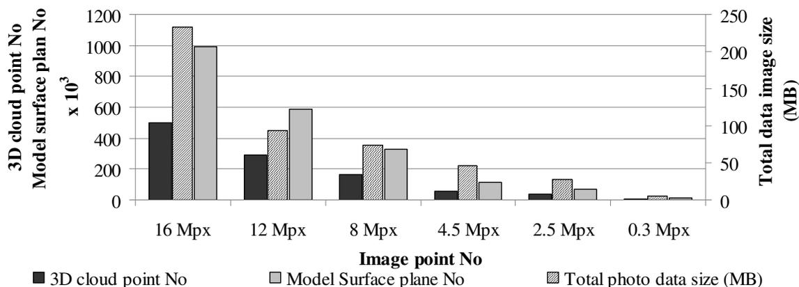
Fig. 4. Graphic dependency of number of 3D cloud points, number of model surface planes and total data image size on number of image points
