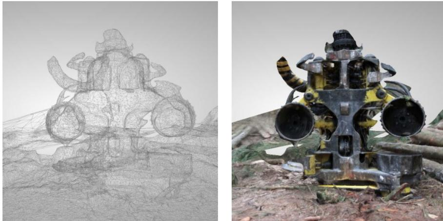
Fig. 2. **Reconstructed 3D model of harvester logging head:** left image – mesh model; right image – model with photorealistic surface
