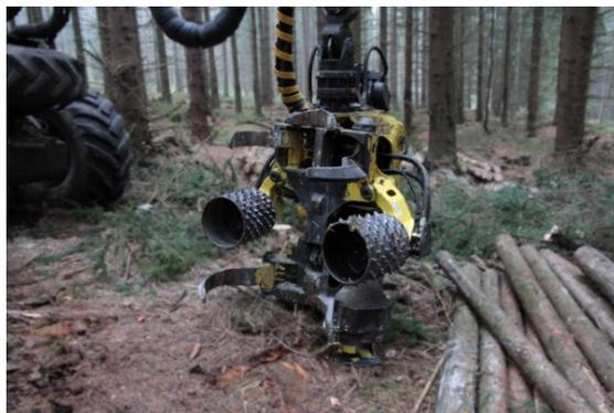
Fig. 1. Photographed logging head of harvester
