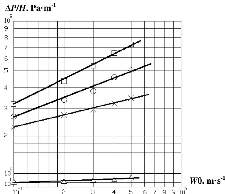
Fig. 3. Dependence of the head loss  $\Delta P/H$  on the flow velocity  $W_0$  for the tested dry packings: □ – mix of wood chips, bark and zeolite granules [1]; ○ – mix of wood chips, bark, granules of zeolite and foam rubber cubes [1]; × – mix of wood chips, bark and foam rubber cubes [1]; Δ – pine cones
