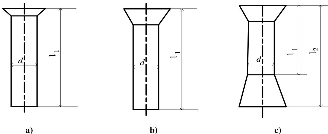
Fig. 1. **Matrix compression channel schemes:** a – cylindrical continuous; b – with creating, calibrating parts; c – with forming, calibrating and relaxation components
