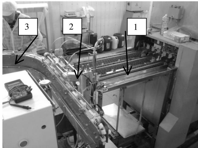
Fig. 1. **Packing line:** 1 – glazing; 2 – transfer; 3 – packaging machines
