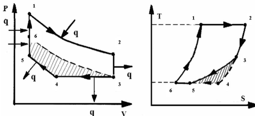
Fig. 3. Ideal Stirling cycle for classical and new Stirling engine modification
