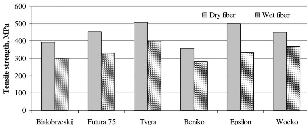
Fig. 4. Tensile strength of hemp fibre depending on hemp varieties for dry and wet fibre
