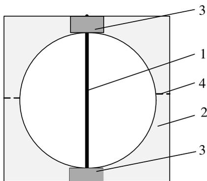
Fig. 1 Fibre sample fixing in the cardboard frame before testing: 1 – fibre sample; 2 – cardboard frame; 3 – strengthen cardboard; 4 – a cut place
