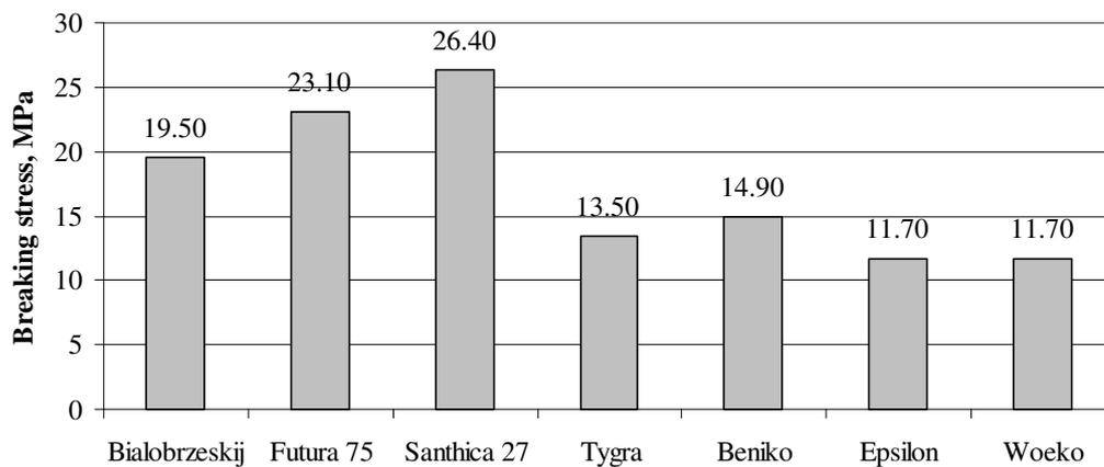
Fig. 7. Longitudinal compressive strength of hemp stems depending on hemp varieties
