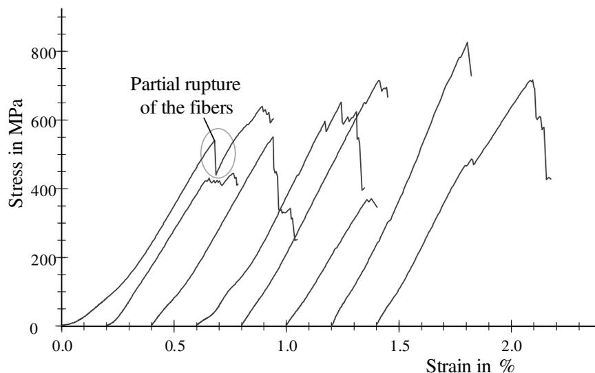
Fig. 3. Hemp fiber specimen rupture curves for different samples of the hemp variety Tygra
