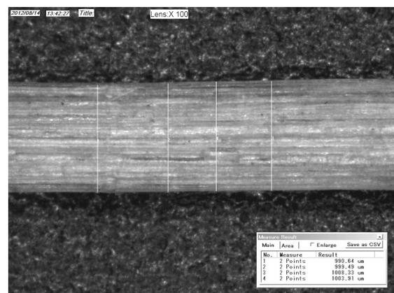
Fig. 2 Fibre sample width measurement with a digital microscope Keyence VHX – 300
