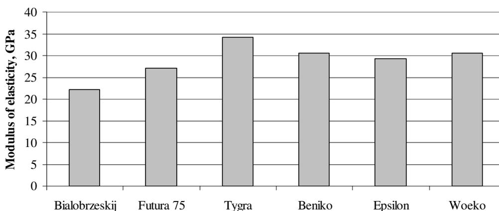
Fig. 6. Modulus of elasticity for different varieties of hemp
