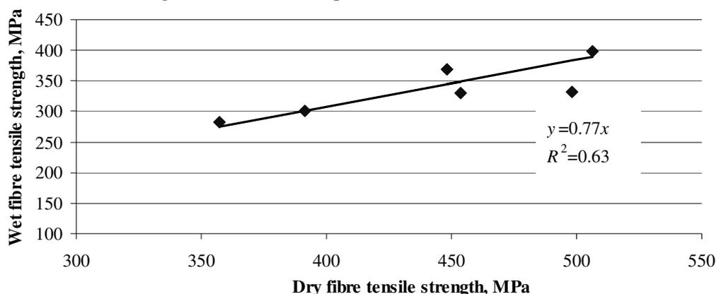
Fig. 5. Wet fibre tensile strength depending on dry fibre tensile strength
