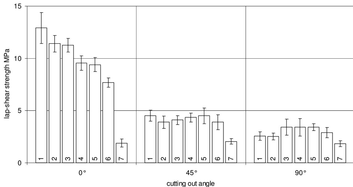
Fig. 2. **Relation between the tensile lap-shear strength and the cutting out angle**
