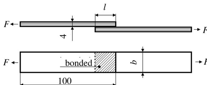
Fig. 1. Tested assembly consisting of two bonded samples
