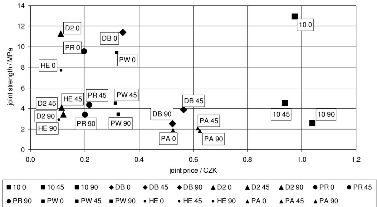
Fig. 3. Strength and price of bonded joints at the use of different adhesives
