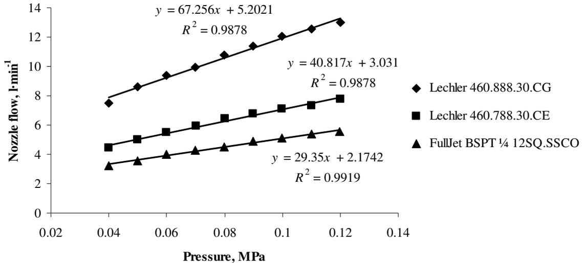
Fig. 2. Measurement of water nozzle flow
