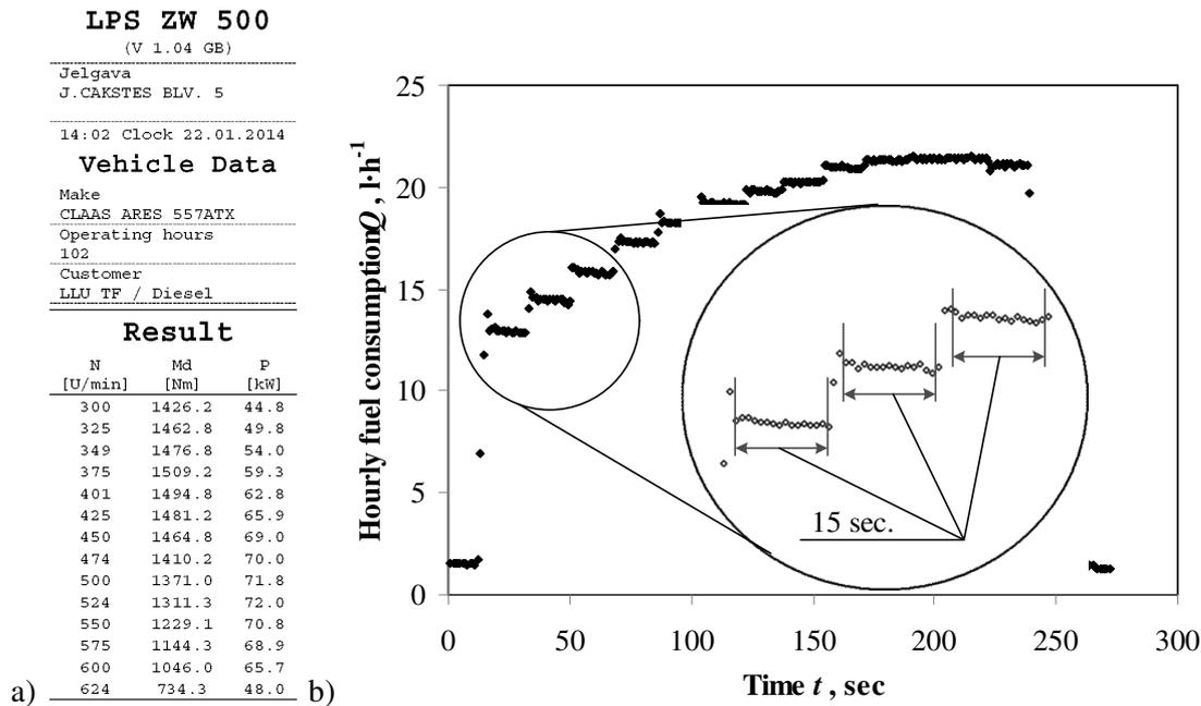
Fig. 2. Examples of raw experiment data: a – printout from the MAHA ZW-500 hand-held terminal; b – raw fuel consumption graph
