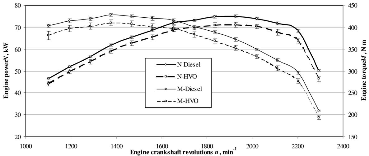
Fig. 3. Engine effective power and torque characteristics
