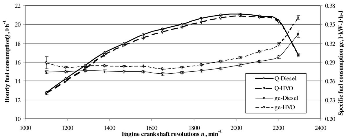
Fig. 4. Fuel consumption characteristics
