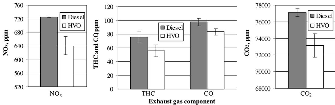
Fig. 5. Content of NO<sub>x</sub>, THC, CO and CO<sub>2</sub> in exhaust gases
