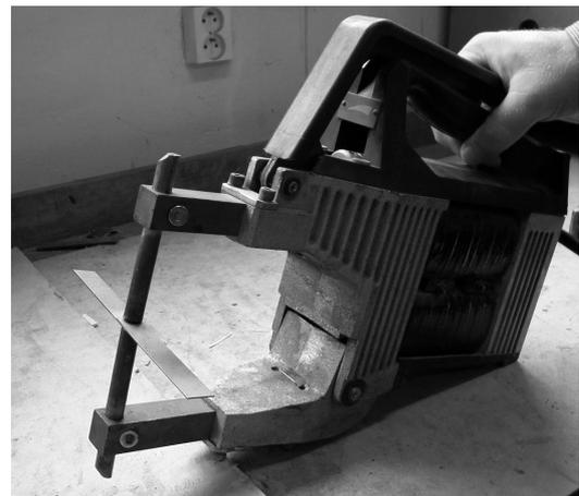
Fig. 2. Welding of steel test samples
