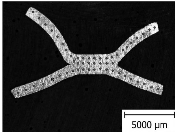
Fig. 5. Scheme of places of microhardness HV0.2 measuring in cut of destroyed bond
