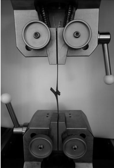
Fig. 3. Destructive testing of test samples
