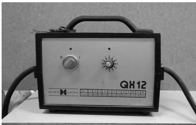
Fig. 1. Regulator of resistance electrode holder – soft mode
