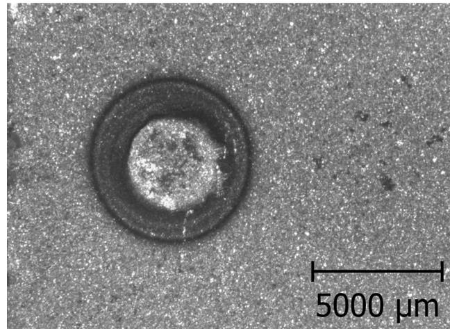
Fig. 4. Weld bond – heat affected zone
