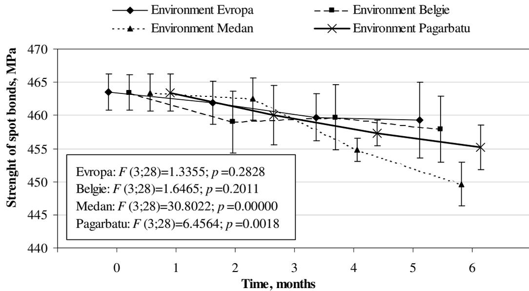
Fig. 6. Influence of time and environment on strength of spot bonds
