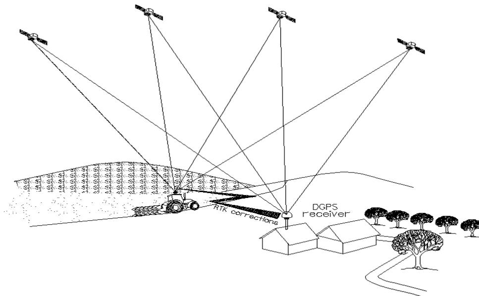
Fig. 1. Precise DGPS data acquisition individual system
