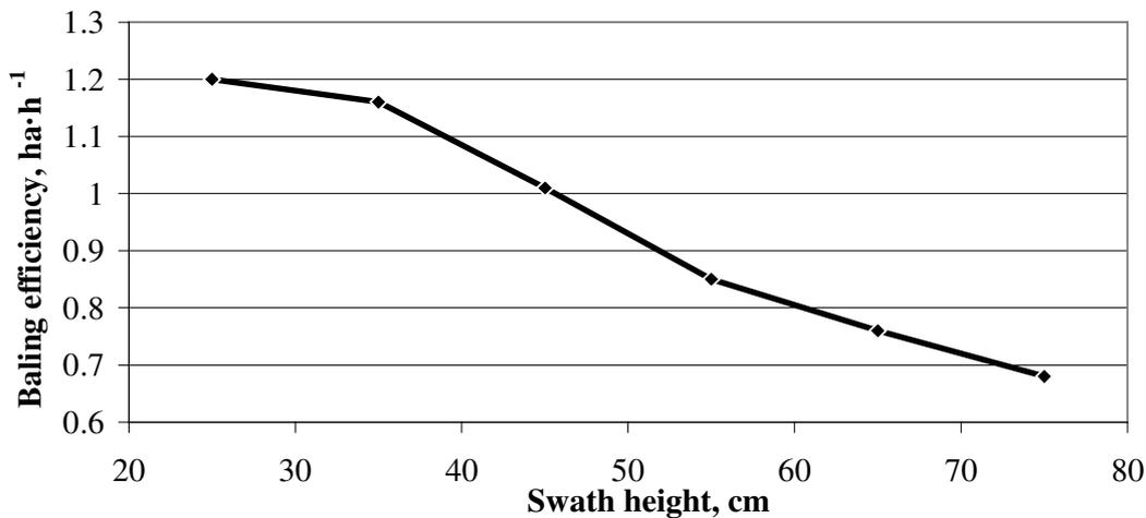
Fig.3. Baling efficiency depending on the height of the shaft
