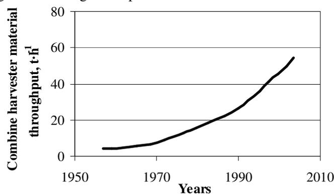
Fig. 1. Increase of material throughput of combine harvester [2]
