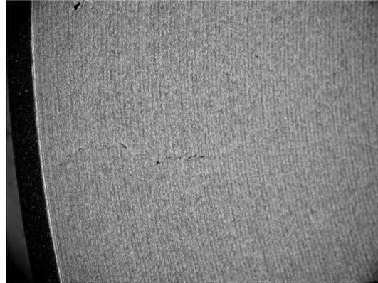
Fig. 2. Crack at the bottom of flange – macro
