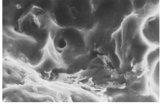
Fig. 5. Transcrystalline ductile fracture – images from electron microscope
