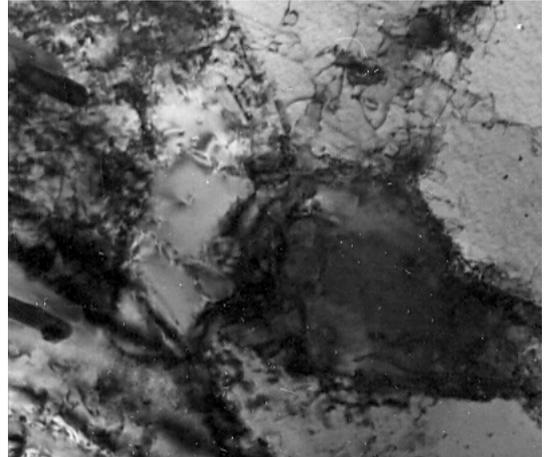
Fig. 7. Substructure in crack – high density of dislocations
