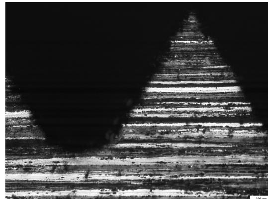
Fig. 4. Microstructure – longitudinal section, Vol. 50x, deformed fibrous structures
