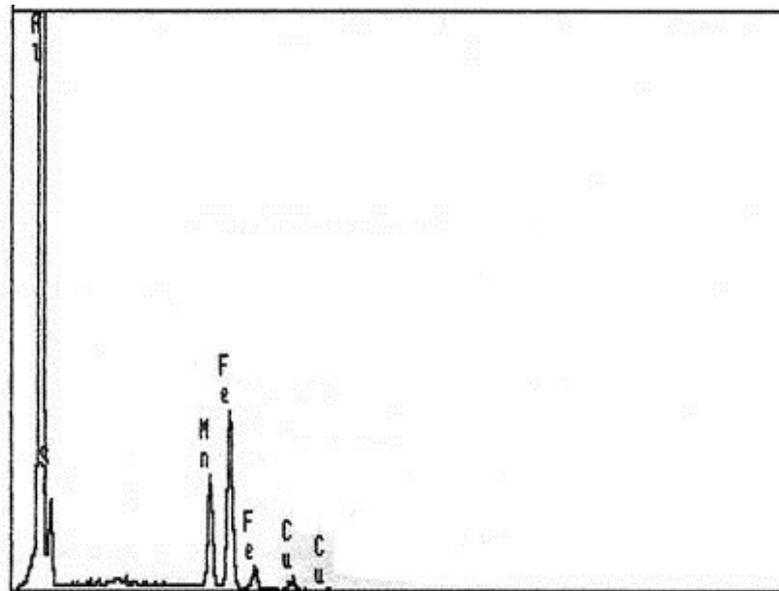
Fig. 8. EDX analysis example of intermetallic particles
