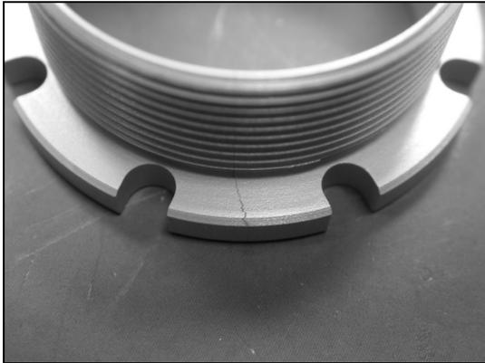
Fig. 1. Product with crack
