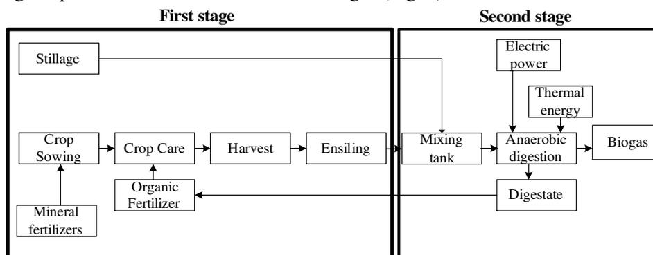
Fig. 1. Technological scheme of biogas production from industrial wastes and energy plants
