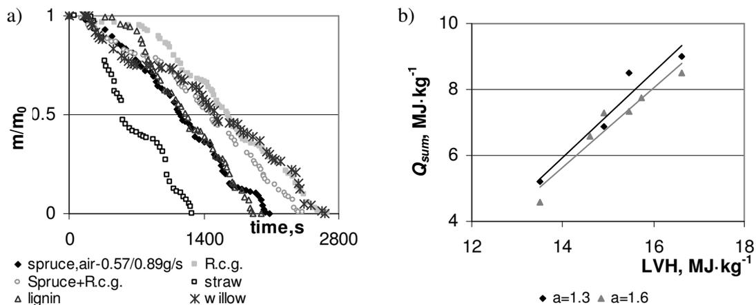
Fig. 1. Time-dependent variations of the weight loss at thermo-chemical conversion of different biomass samples (a), and correlation between the produced heat energy and LHV (Lower Heating Value) of the biomass pellets at different air excess “a” factors (b)
