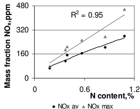
Fig. 2. Correlation between the nitrogen content in biomass pellets and the mass fraction of NO<sub>x</sub> emission in the products
