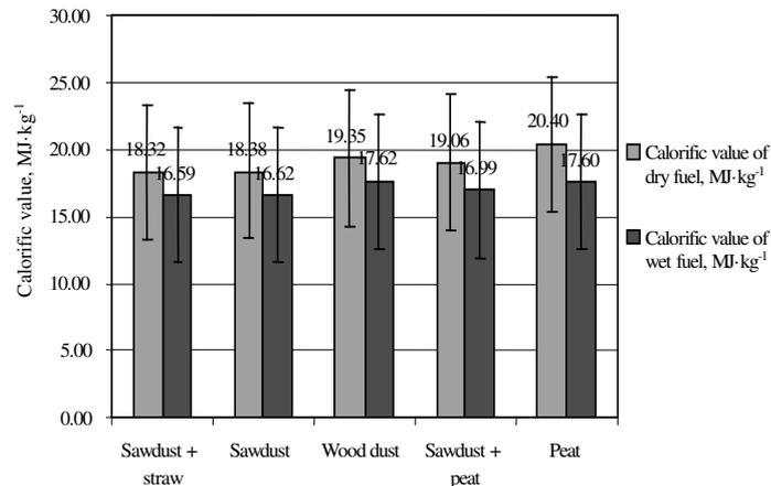
Fig. 6. Calorific value of dry and wet fuel,  $\text{MJ}\cdot\text{kg}^{-1}$
