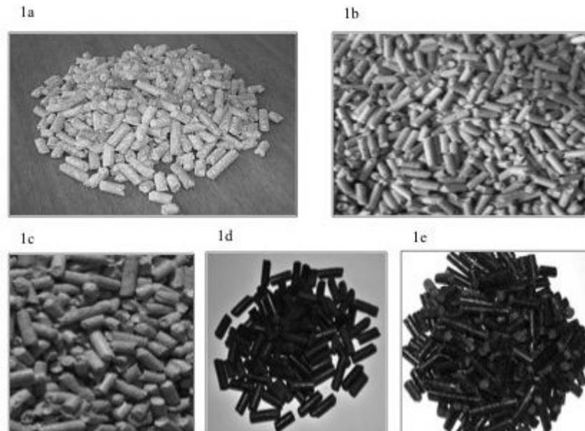
Fig. 1. Sawdust + straw pellets (1a); homogeneous sawdust pellets (1b); homogeneous wood dust pellets (1c); sawdust + peat pellets (1d); homogeneous peat pellets (1e)
