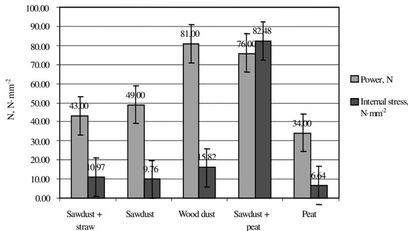
Fig. 7. Average internal stress and load force
