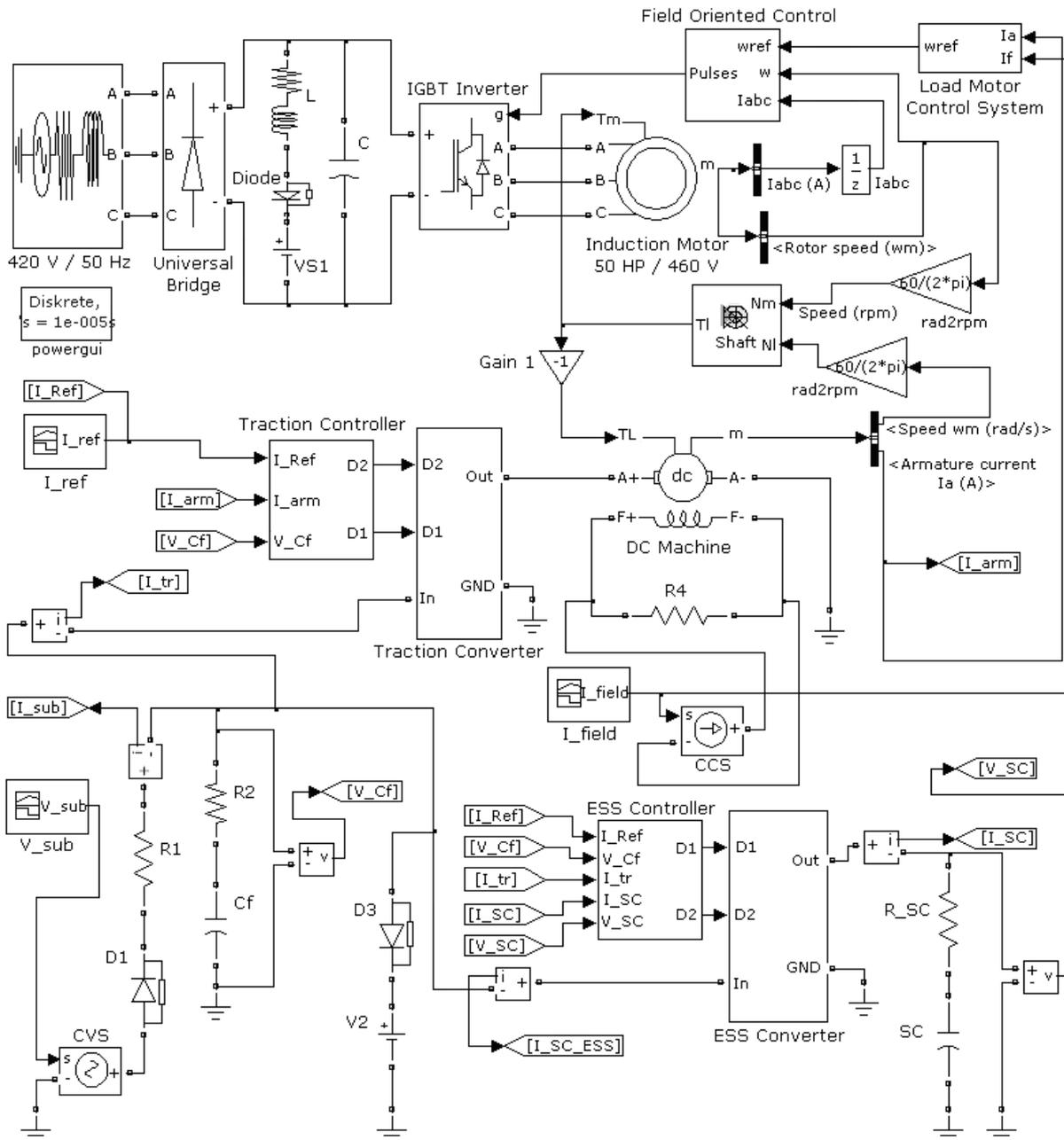
Fig. 2. Simplified Matlab/Simulink model of the traction drive test bench
