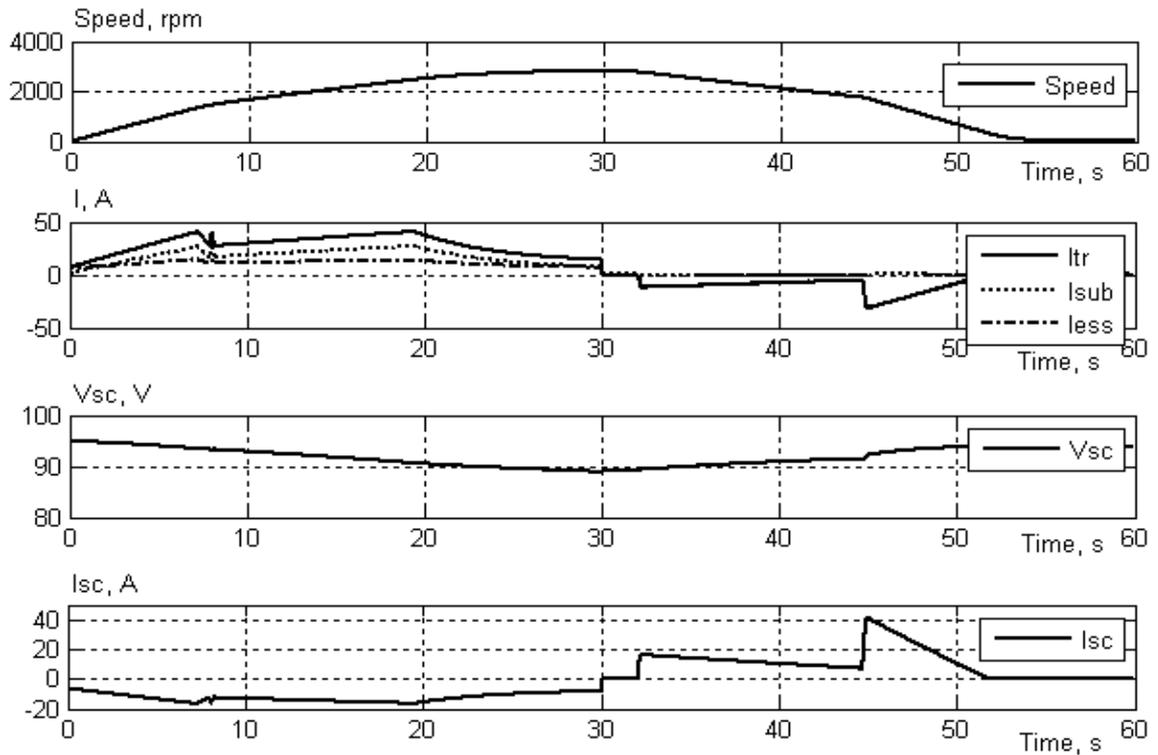
Fig. 3. **Simulation diagram at correct choice of excitation current value:**  $I_{tr}$  – traction current;  $I_{sub}$  – substation current;  $I_{ess}$  – ESS current;  $I_{ref}$  – armature current reference;  $I_{arm}$  – armature current;  $V_{sc}$  – supercapacitor voltage;  $I_{sc}$  – supercapacitor current
