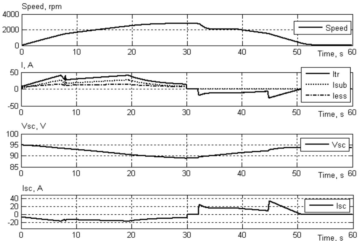
Fig. 4. **Simulation diagram at incorrect choice of excitation current value:**  $I_{tr}$  – traction current;  $I_{sub}$  – substation current;  $I_{ess}$  – ESS current;  $I_{ref}$  – armature current reference;  $I_{arm}$  – armature current;  $V_{sc}$  – supercapacitor voltage;  $I_{sc}$  – supercapacitor current
