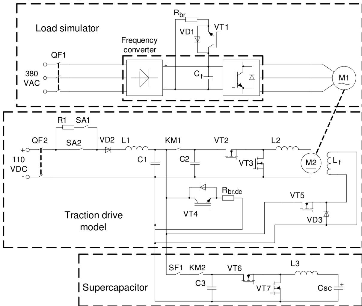
Fig. 1. Schematics of the traction drive test bench with supercapacitor energy storage system
