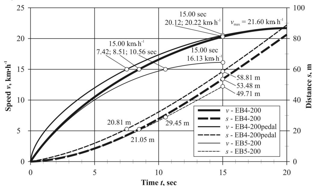
Fig. 5. Acceleration characteristics testing EB4-200 and EB5-200 electric bicycles
