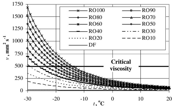
Fig. 7. Fuel blend viscosity depending on ambient temperature
