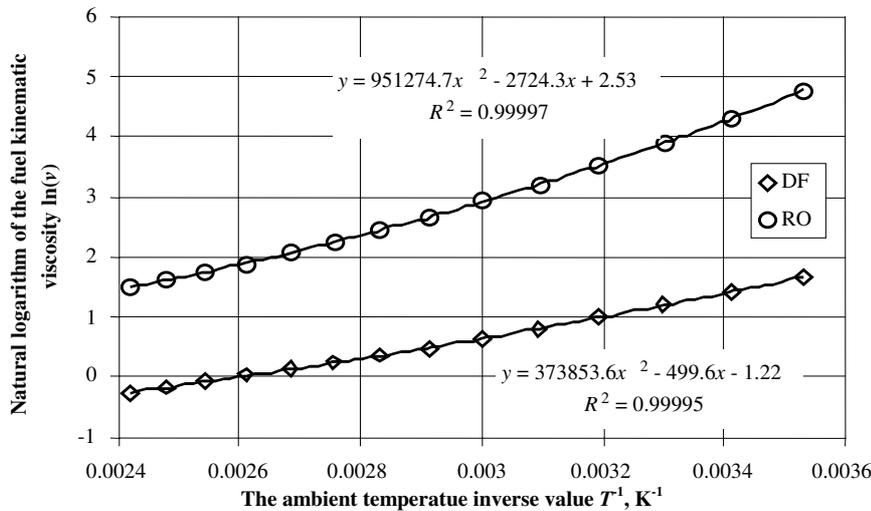
Fig. 2. Determination of coefficients for calculating of fuel kinematic viscosity
