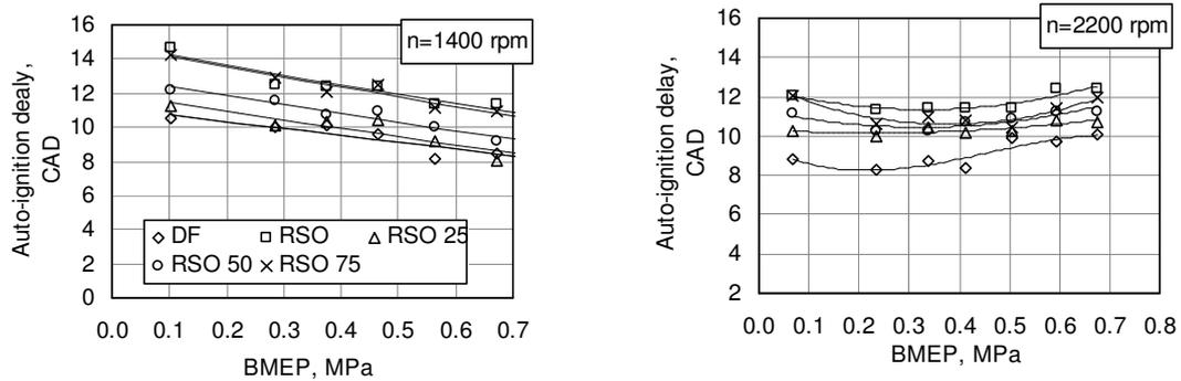
Fig. 1. Dependency of auto-ignition delay on engine load and rapeseed oil amount in the fuel
