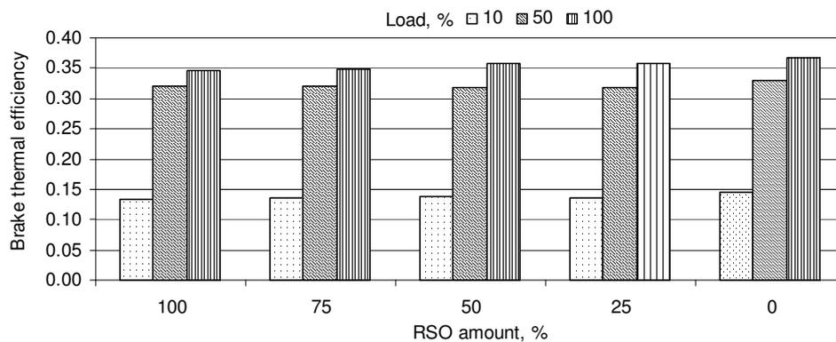
Fig. 4. Influence of the amount of RSO in fuel and engine running mode on the brake thermal efficiency
