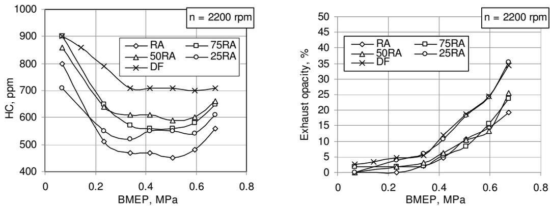
Fig. 6. Influence of the amount of RSO in fuel on HC emissions and exhaust opacity
