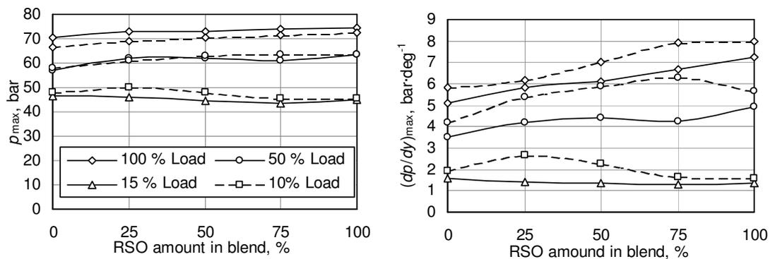
Fig. 2. In-cylinder pressure peak ( $p_{max}$ ) and maximum cylinder pressure gradient ( $(dp/d\phi)_{max}$ ) as functions of RSO amount in fuel: —  $n = 1400 \text{ min}^{-1}$ ; ---  $n = 2200 \text{ min}^{-1}$
