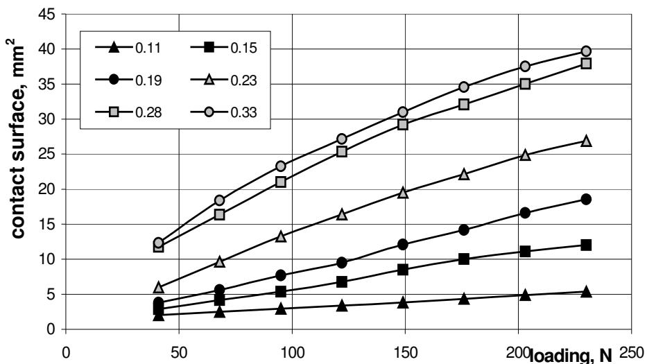
**Fig. 2. Change of the unit contact surface depending on the load at various water content levels in Jubilatka species of beans**
