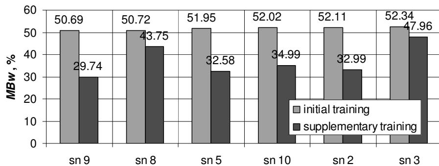
**Fig. 3.  $MBw$  measure values for the RFB and MLP networks after supplementary training (validation data)**
