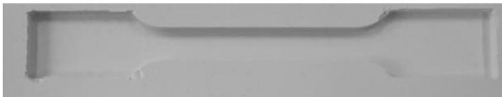
Fig. 1. Mould for casting the test specimens
