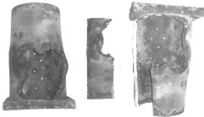
Fig. 1. Body of gutted by fire pellet torch before and after cutting out the sample for the research
