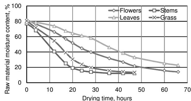
Fig. 2. Dynamics of herbal raw material (*Echinacea purpurea* L. Moench) drying in a thick still mound
