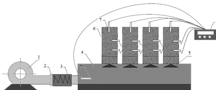
Fig. 1. **Basic scheme of a test-bench for material drying in a still thick layer:** 1 – fan; 2 – flexible flange; 3 – electric heater; 4 – air flow distribution manifold; 5 – hatches; 6 – ventilated containers; filled with herbal raw material; 7 – temperature and relative humidity sensors; 8 – data logger Almemo
