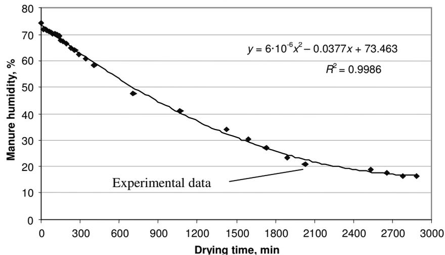
Fig. 3. Manure humidity changes by convection with air speed at top  $0.27 \text{ m}\cdot\text{s}^{-1}$
