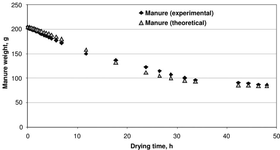
Fig. 4. Manure weight changes during the drying process by convection with air speed at top  $0.27 \text{ m}\cdot\text{s}^{-1}$
