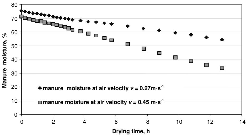
Fig. 5. Manure moisture changes during the drying process by convection with air speeds at top  $0.27 \text{ m}\cdot\text{s}^{-1}$  and  $0.45 \text{ m}\cdot\text{s}^{-1}$
