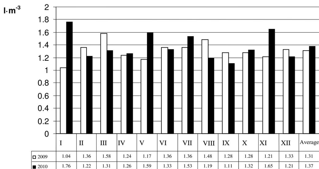
**Fig. 5. Harwarder “Ponsse BD” fuel consumption per m<sup>3</sup> of harvested timber, 2009-2010**
