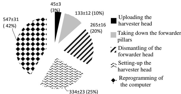
Fig. 1. Stages of the forwarder into harvester transformation (s)
