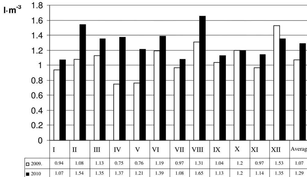
Fig. 6. Harwarder “Ponsse BD” fuel consumption per m<sup>3</sup> of extracted timber, 2009-2010
