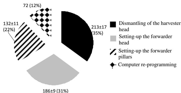
Fig. 2. Stages of the harvester into forwarder transformation (s)
