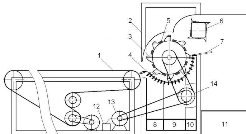
Fig. 1. **Scheme of the stationary corn ear threshing unit:** 1 – corn ear belt-feeder; 2 – frame of the threshing unit; 3 – threshing cylinder; 4 – concave; 5 – additional ballast bars; 6 – back beater; 7 – transition grate; 8, 9, 10 – tanks for collecting grain; 11 – collection tank; 12 – devices for measuring electric current, voltage and power; 13 – electric motor; 14 – variator
