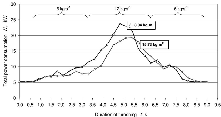
Fig. 6. Variation of power consumption during corn ear threshing at inconsistent feed rate, when operating cylinders with different moments of inertia
