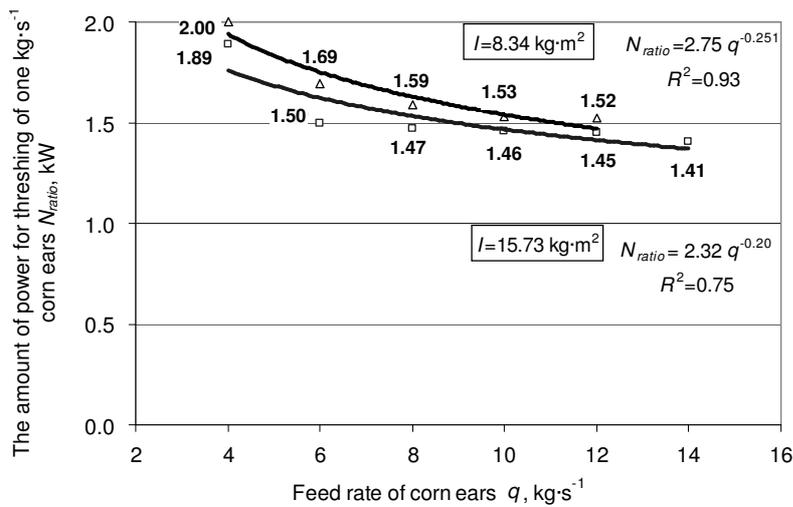
Fig. 4. Effect of the feed rate  $q$  on the amount of power required for threshing of one  $\text{kg}\cdot\text{s}^{-1}$  of corn ears  $N_{ratio}$  while operating threshing cylinders with different moments of inertia  $I$
