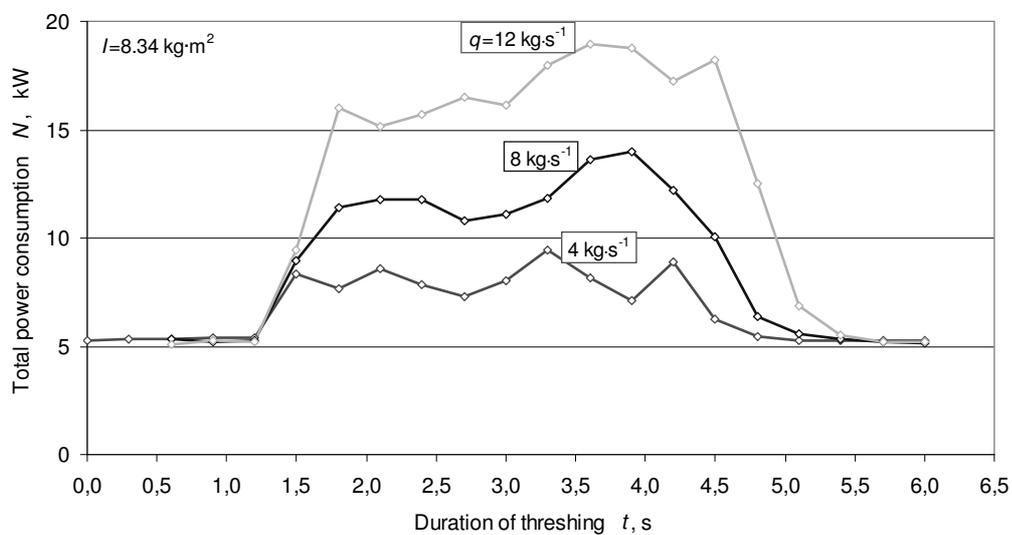
Fig. 2. Variation of power consumption under different corn feed rate with the moment of inertia of the threshing cylinder  $I = 8.34 \text{ kg}\cdot\text{m}^2$  (cylinder mass  $m = 204.2 \text{ kg}$ )
