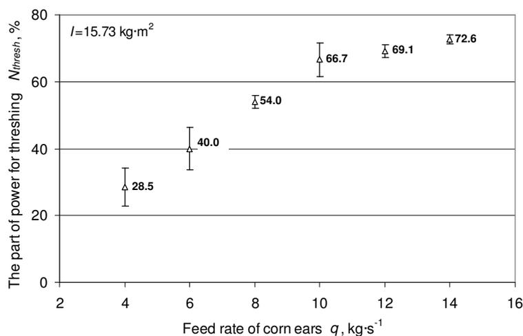
Fig. 5. Effect of the corn feed rate on the part of power required for only threshing corn ears ( $I = 15.73 \text{ kg}\cdot\text{m}^2$ , cylinder mass  $m = 320.2 \text{ kg}$ )
