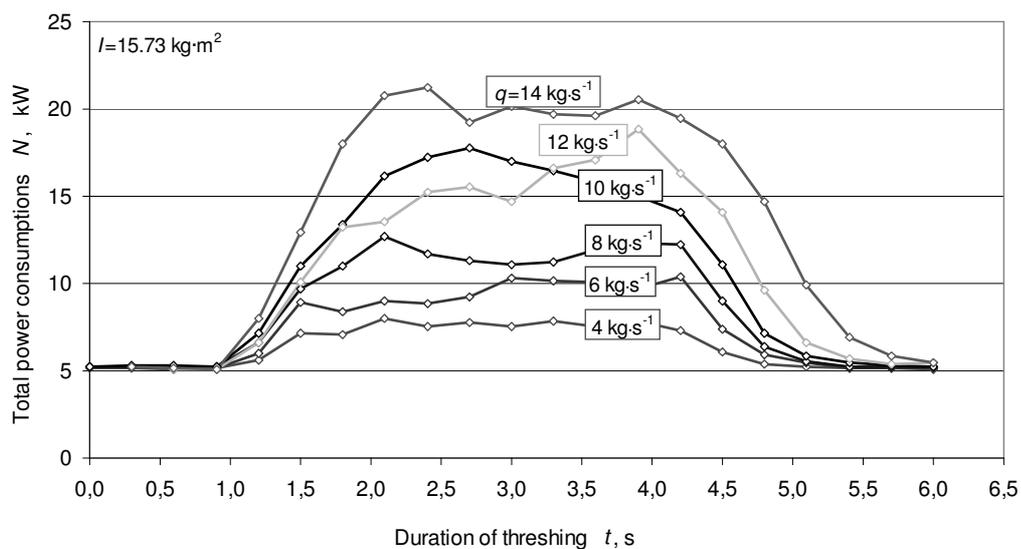
Fig. 3. Variation of power consumption under different corn feed rate with the moment of inertia of the threshing cylinder  $I = 15.73 \text{ kg}\cdot\text{m}^2$  (cylinder mass  $m = 320.2 \text{ kg}$ )
