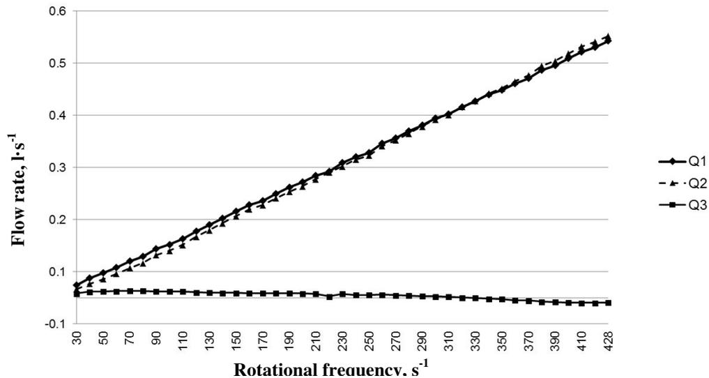
Fig. 5. Graph of dependency of hydraulic oil flow on cutting disc rotational frequency: Q1 – hydraulic oil flow in pressure line; Q2 – hydraulic oil flow in drain line; Q3 – calculated flow of leakage fluid
