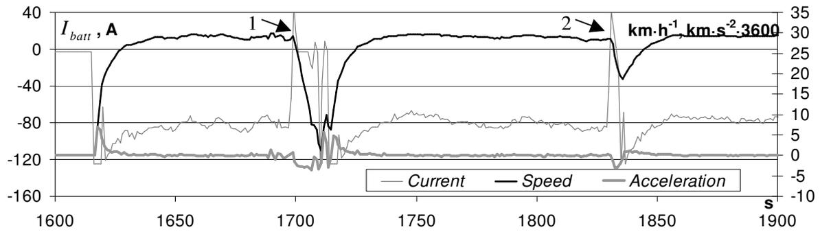
Fig. 4. Battery current dependence on acceleration
