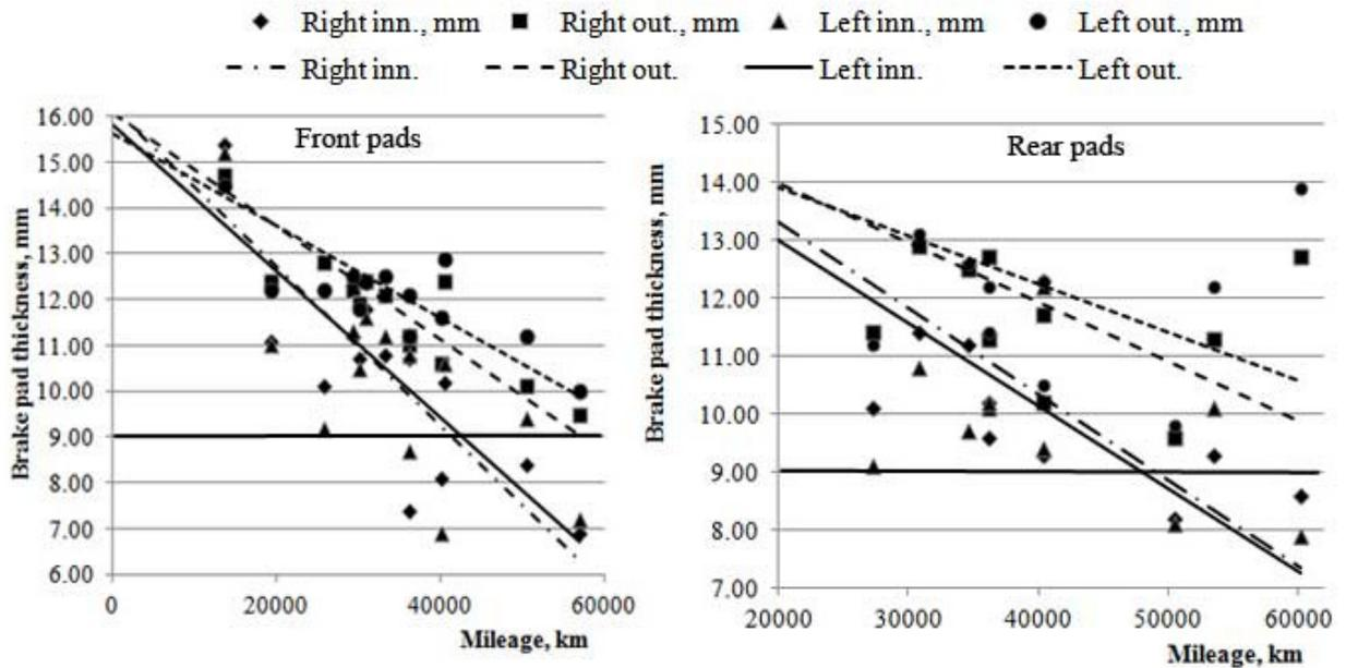
Fig. 1. Brake pad wear data, Renault Traffic II
