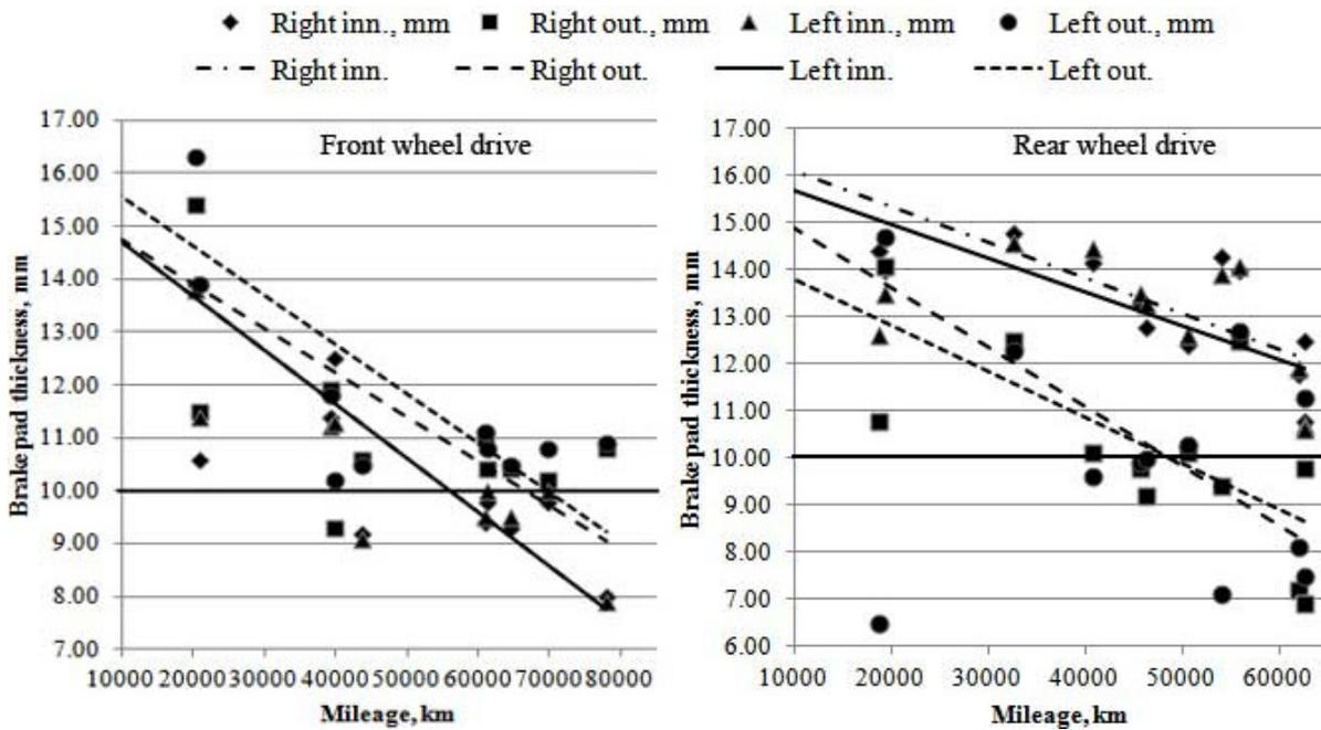
Fig. 3. Brake pad wear data, Renault Master III, rear pads
