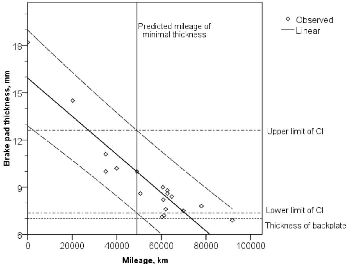
Fig. 4. Results of prediction, Renault Master III, front inner pad
