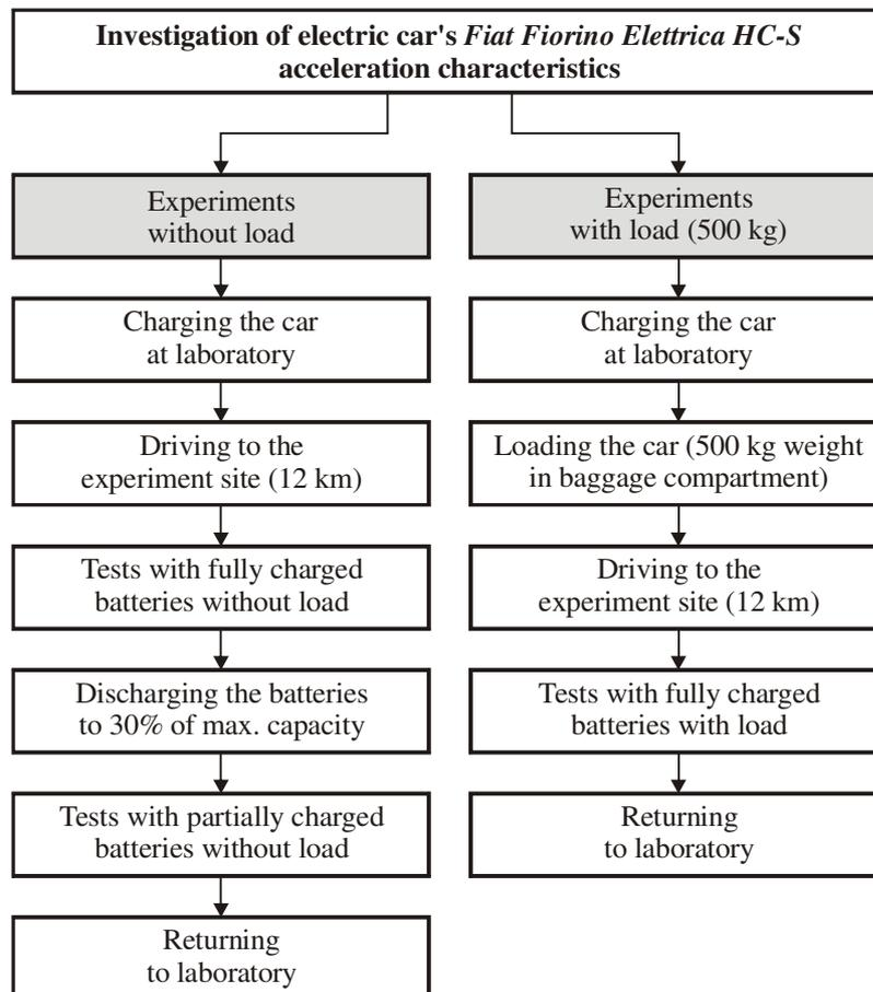
Fig. 2. Block diagram of experiments
