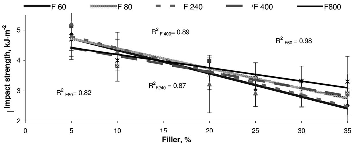
Fig. 2. Influence of filler share in matrix on impact strength of polymeric particle composites with waste-corundum-based filler
