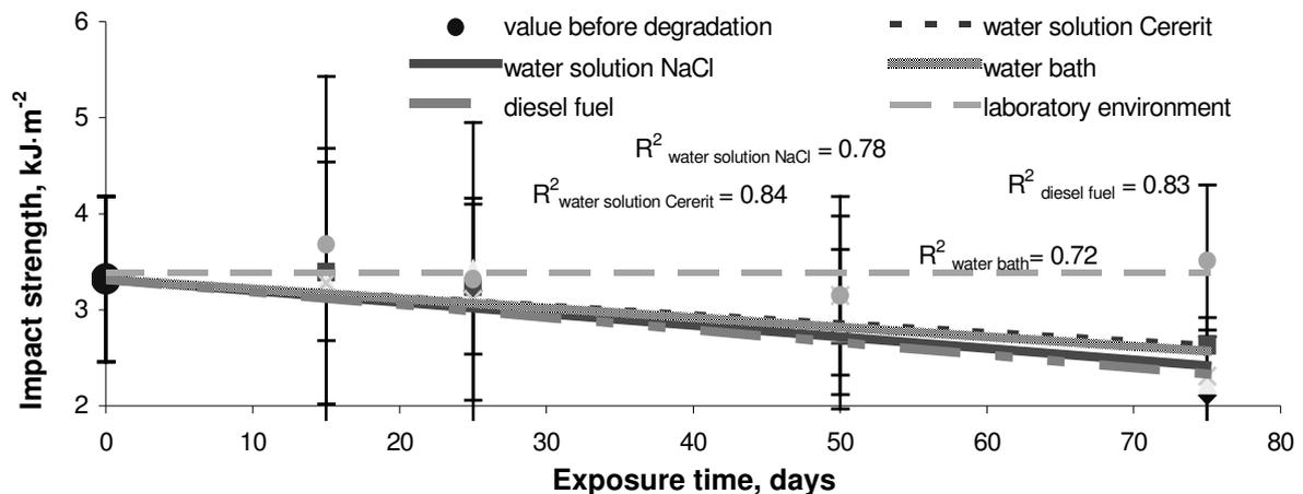
Fig. 3. Influence of degradation on impact strength
