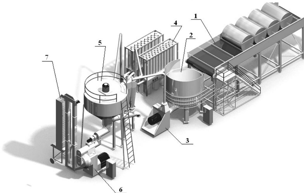
Fig. 1. **Technological line for straw pelleting:** 1 – conveyor, 2 – shredder, 3 – mill, 4 – air cleaning system, 5 – hopper for chopped material, 6 – pelleting press, 7 - cooler
