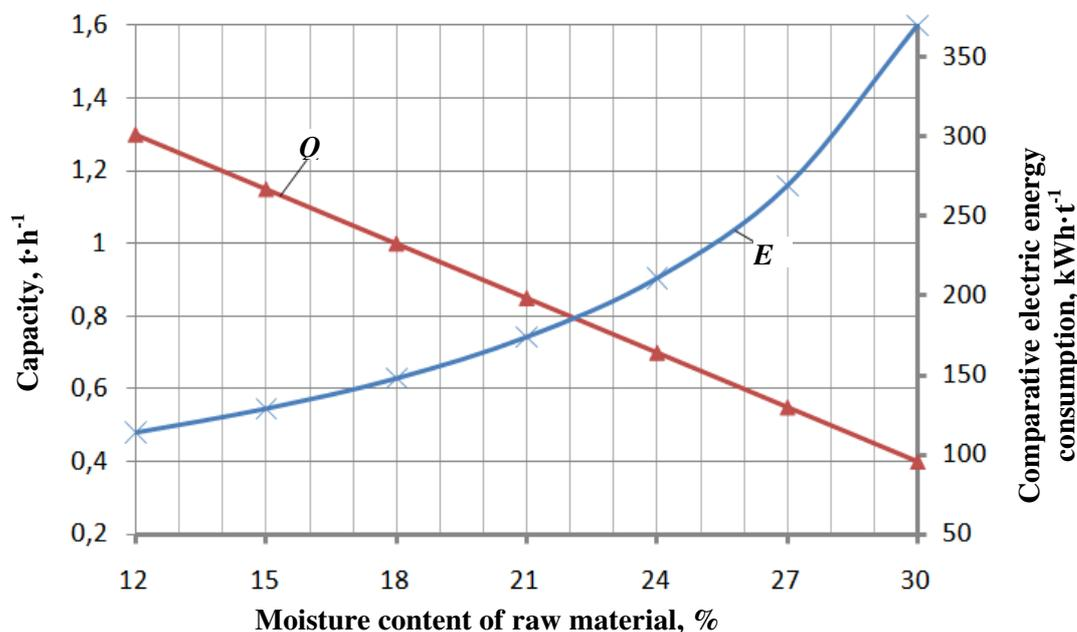
Fig. 3. Variation of the technological line capacity and energy consumption:  $Q$  – capacity of technological line subject to moisture content of raw material, t·h<sup>-1</sup>,  $E$  – variation of comparative electric energy consumption subject to moisture content of raw material, kWh·t<sup>-1</sup>
