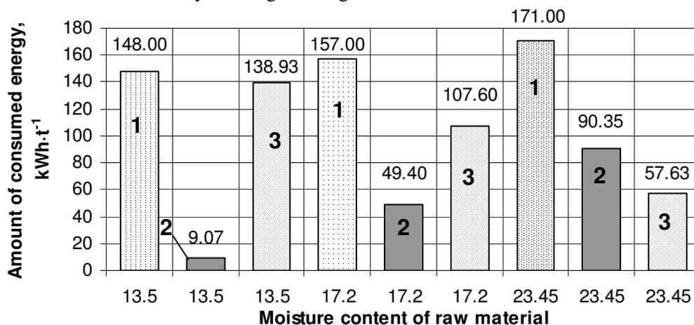
Fig. 5. Kinetics of energy consumption at changing straw moisture content: 1 – energy consumed in pellet production; 2 – energy consumed in moisture evaporation; 3 – energy used in mechanical processes of pellet production
