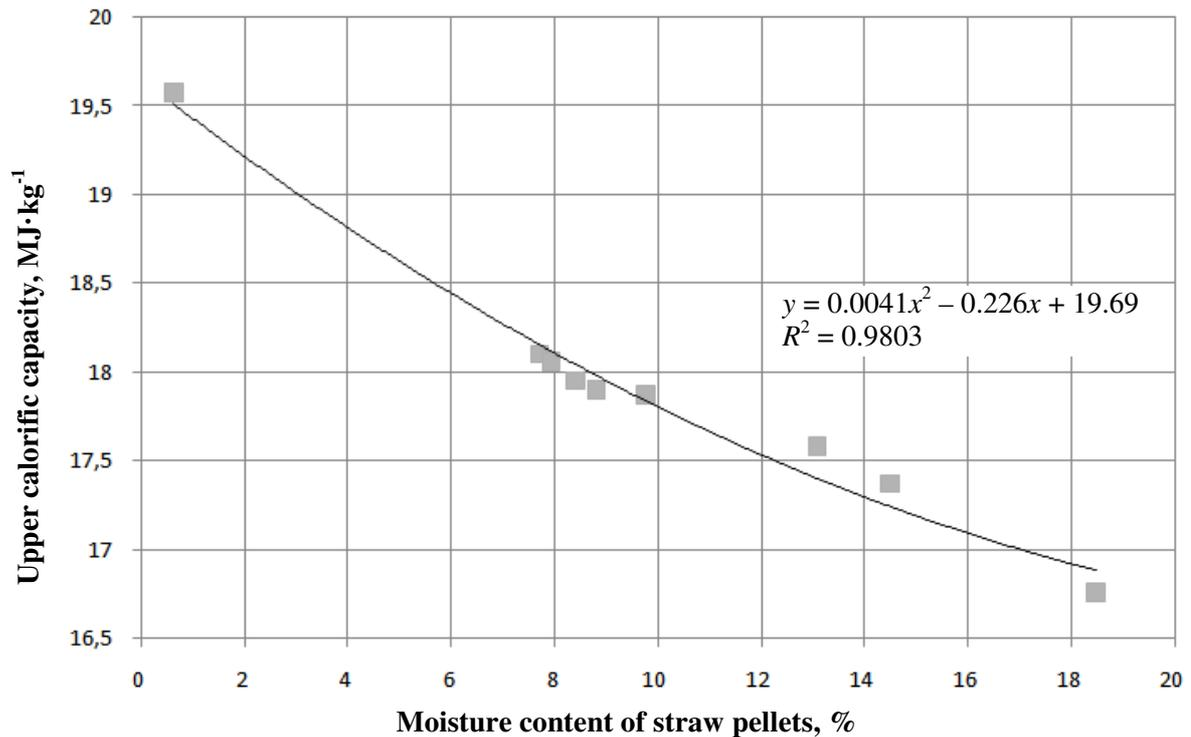
Fig. 4. Variation of straw pellet calorific capacity
