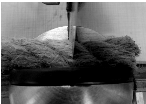
Fig. 9. Strongly twisted hemp rope cutting
