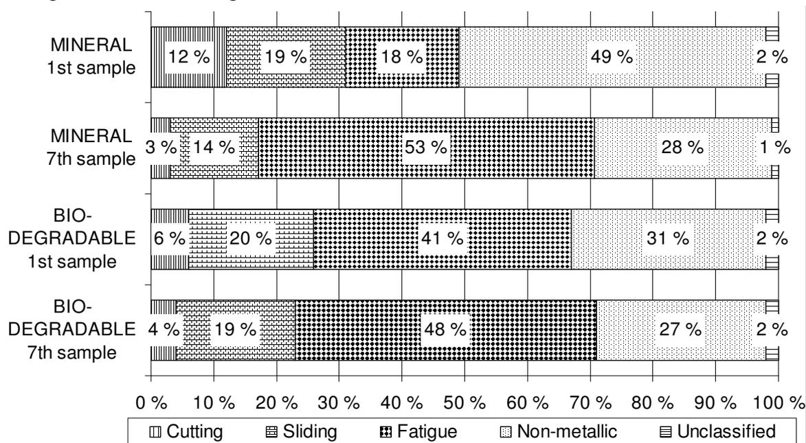
**Fig. 3. Percentage fraction of different particles in transmission oil samples**
