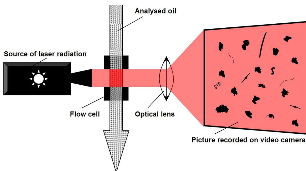
Fig. 2. Principle of LNF analysis [6]
