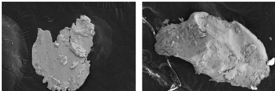
Fig. 1. Shape of fatigue particle [2]
