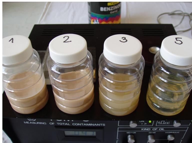
Fig. 4. Hydraulic fluid samples contaminated with water
