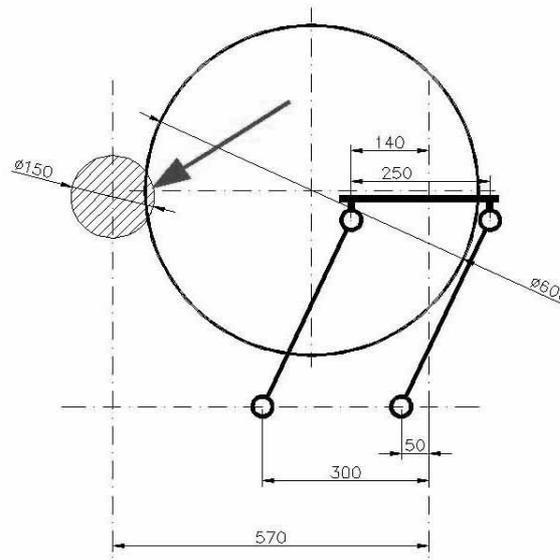
Fig. 3. Kinematics of Wallner interaxle carrier – maximum deflection of cutting disc
