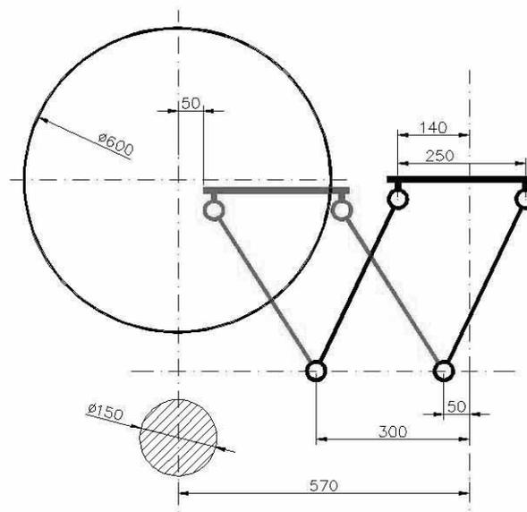
Fig. 2. Kinematics of Wallner interaxle carrier – cutting disc operating position
