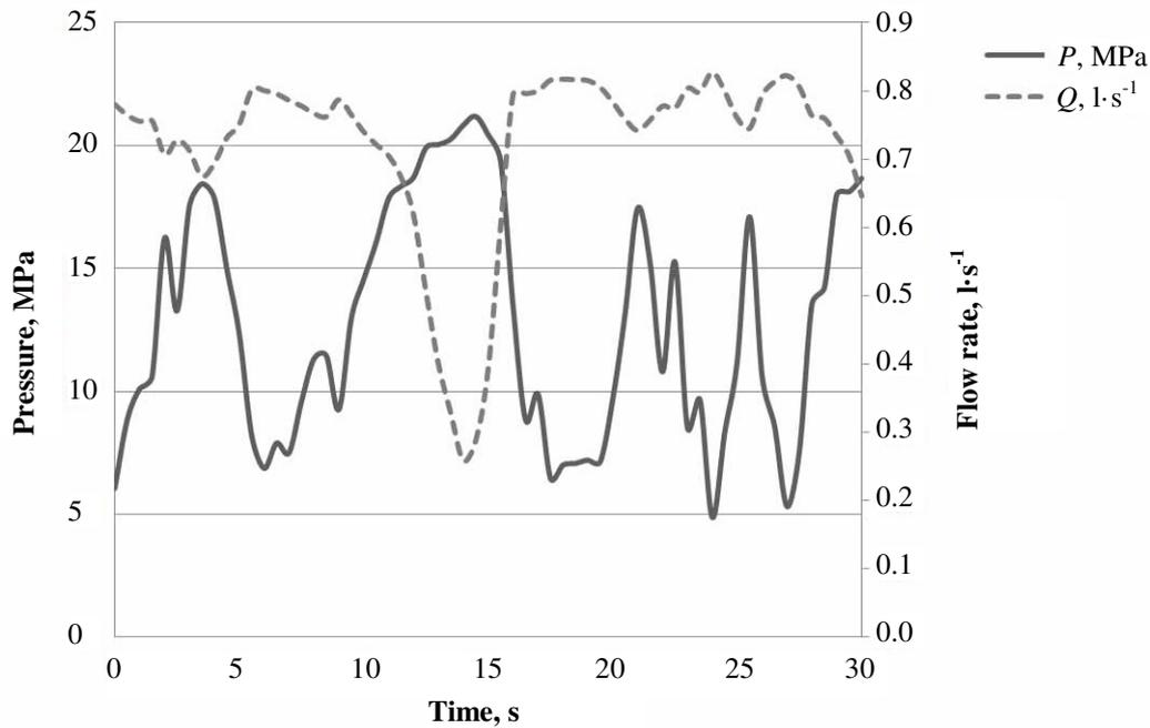
Fig. 4. Graph of dependency of hydraulic oil pressure and flow on time
