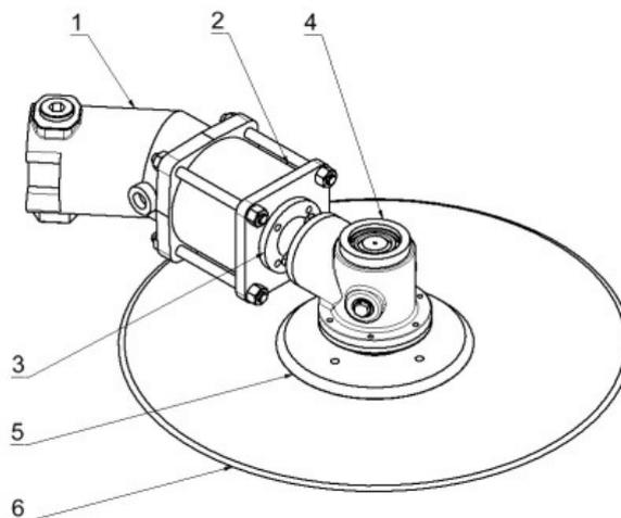
Fig. 5. **Rear transmission with hydromotor:** 1 – axial piston hydromotor; 2 – clutch; 3 – extension; 4 – angular gear; 5 – carrier; 6 – cutting disc
