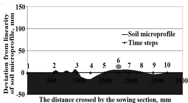
Fig. 6. Arrangement mode of time steps on surface covered by sowing section
