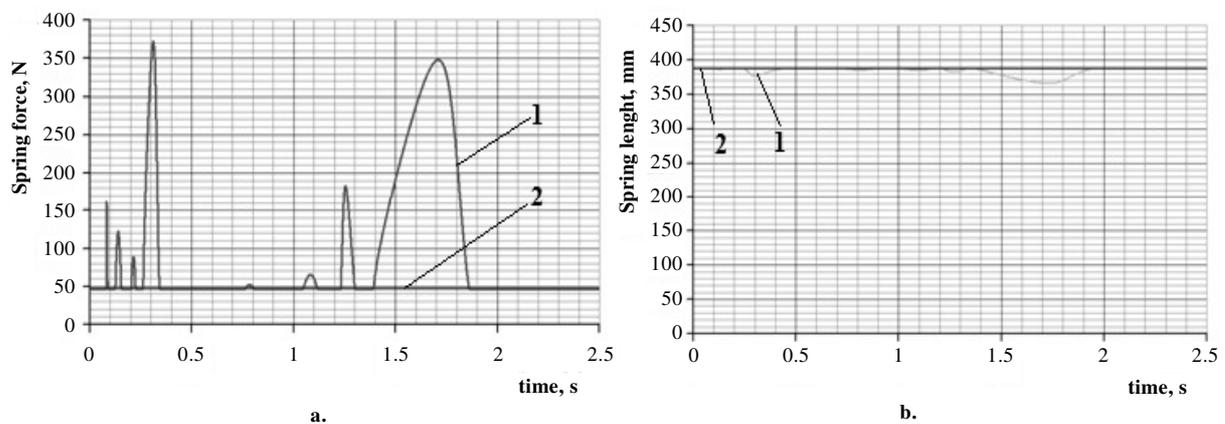
Fig. 5. Diagram of variation in time of force from spring (a) and spring length (b), for two profiles of soil surface: 1 – soil with smooth surface; 2 – soil with unevenness
