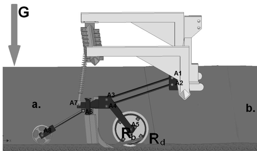
Fig. 2. **Dynamic model of working section of grassland oversowing machine:**
