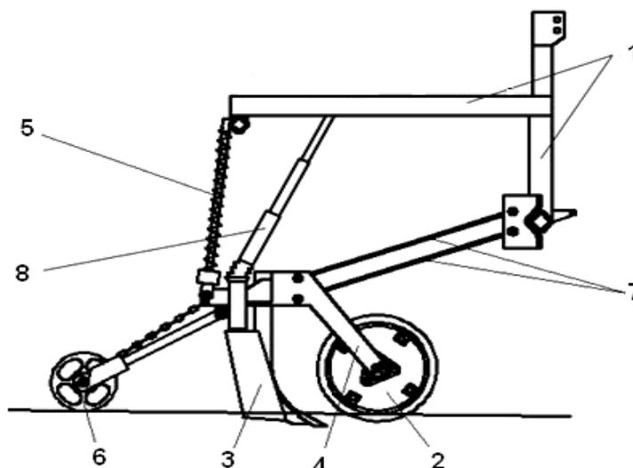
Fig. 1. Constructive scheme of working section of grassland oversowing machine [3]:
