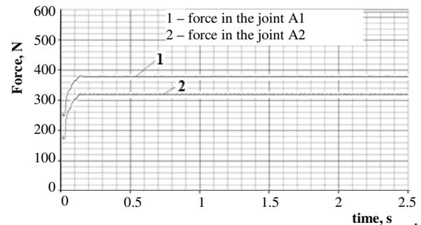
Fig. 4. Diagram of variation in time of forces from A1 and A2 joints of parallelogram mechanism (s. Fig. 2), for soil with smooth surface
