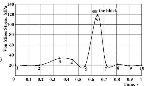
Fig. 7. Curve of maximum stress in top bar of parallelogram mechanism
