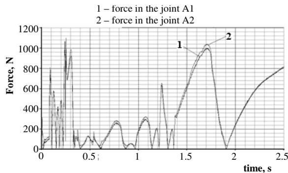
Fig. 3. Diagram of variation in time of forces from A1 and A2 joints of parallelogram mechanism (s. Fig. 2), for soil with unevenness
