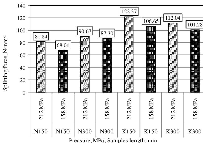
Fig. 9. Specific splitting force of reed and hemp stalk particles, N – reed, K – hemp
