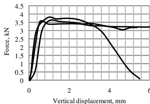
Fig. 1. Typical compressive load-displacement curves of hemp stem
