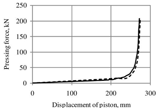
Fig. 2. Typical briquetting force-displacement curves of hemp stem, particle length 150 mm
