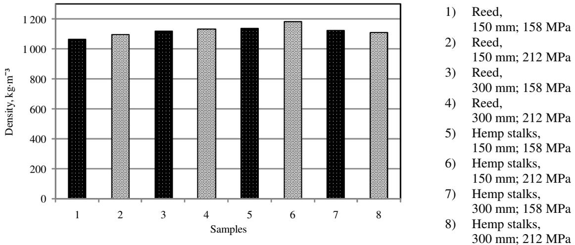
Fig. 7. Change of briquette density depending on briquetting pressure and particle length for reed and hemp stalks
