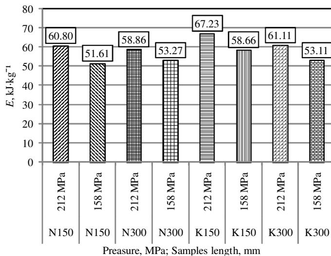
Fig. 8. Briquetting energy of arranged reed and hemp stalk particles, N – reed, K – hemp
