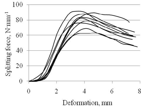
Fig. 4. **Force – deformation diagram for not flattened reed stalks, 300 mm length**
