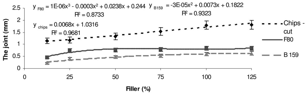
Fig. 2. Joint thickness
