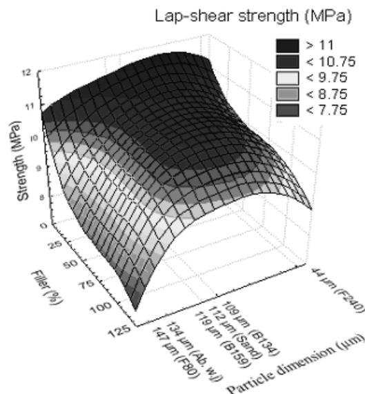
Fig. 3. Lap-shear strength
