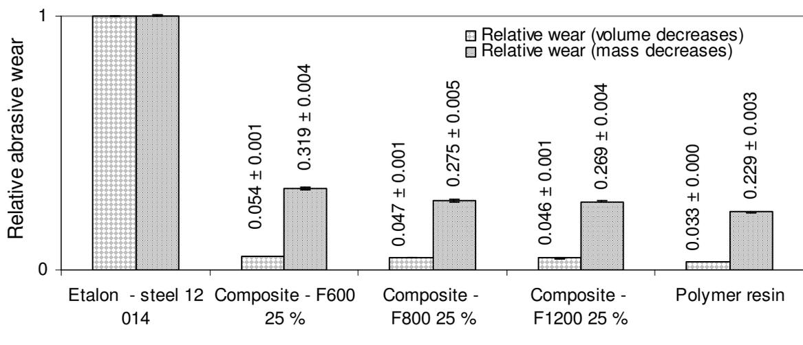
Fig. 5. Comparison of resistance against abrasive wear
