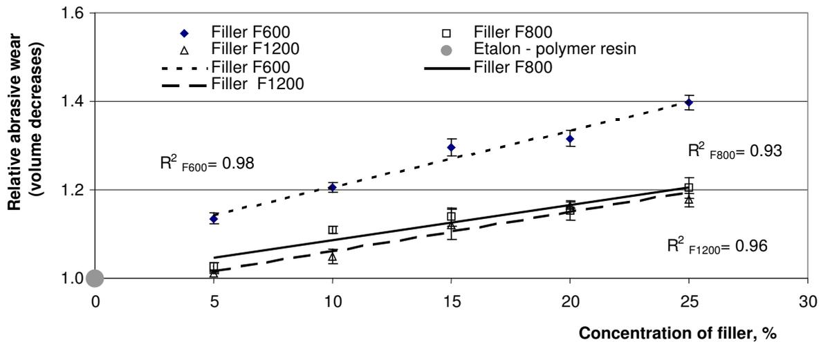
Fig. 4. Influence of polymeric particle composite concentration and granularity to wear
