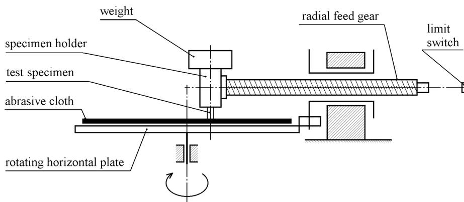
Fig. 2. Scheme of equipment for testing abrasive wear [15]
