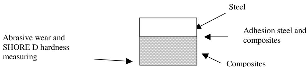
Fig. 1. Tested specimen for testing abrasive wear and SHORE D hardness
