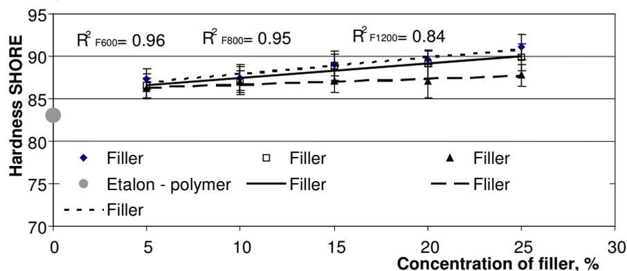
Fig. 3. Influence of polymeric particle composite filler concentration and granularity to hardness
