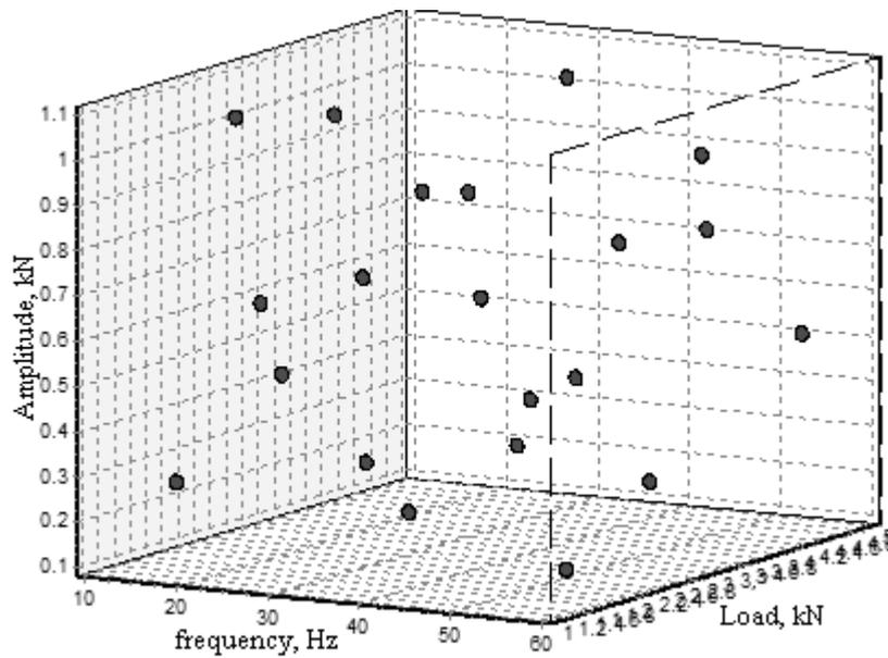
Fig. 1. Mean Square Error Latin hypercube design
